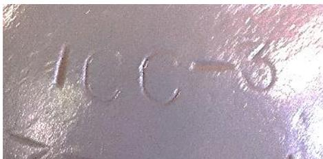
**Figure 1 - Example of VALID ICC-3 marking**
