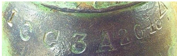
**Figure 2 – Example of an Altered ICC-3 Marking - CONDEMN**
